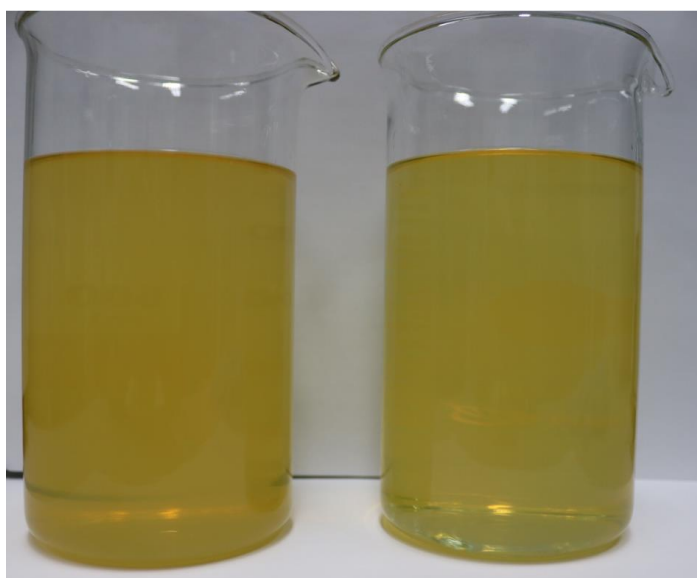
Figure 3.3 Ether surrogate unfiltered (left) and filtered (right).
