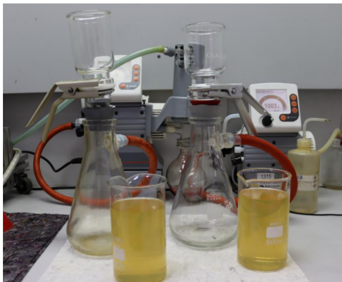
Figure 3.2 Overview of the double set-up applied for fuel filtration.
