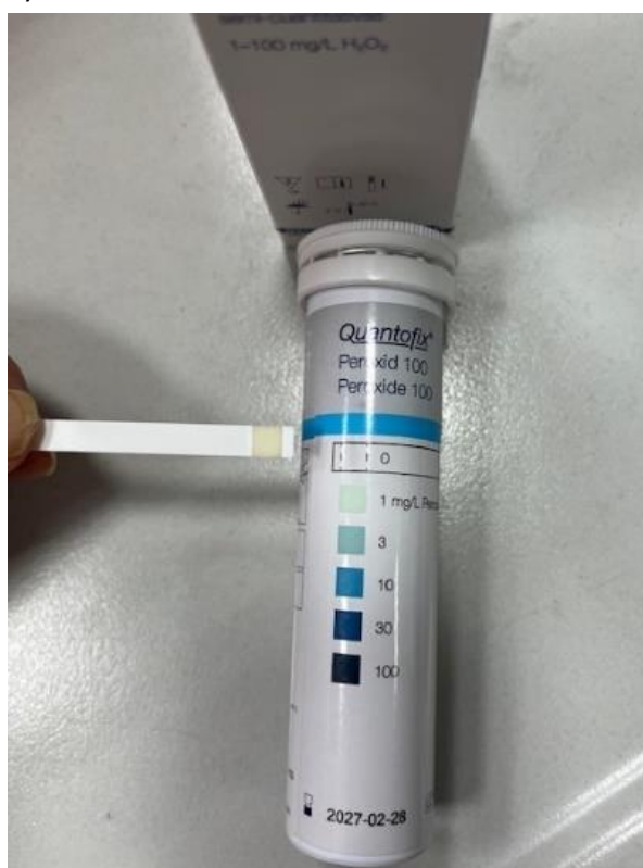
Figure 3.6 Result of the peroxide test on the filtered ether surrogate.
