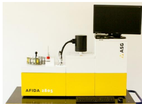
Figure 2.1 Advanced Fuel Ignition Delay Analyzer (AFIDA) device (right) and operating principle (left).
