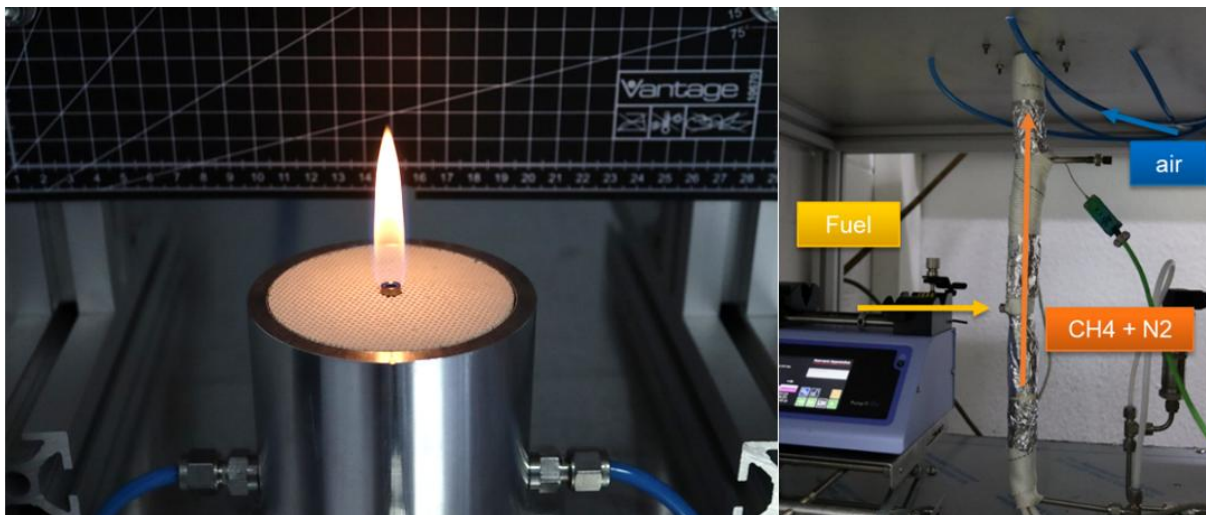
Figure 2.2 Yale-Coflow burner (chimney not attached) with established flame (left) and dopant dosing unit and heated fuel line underneath the burner (right)
