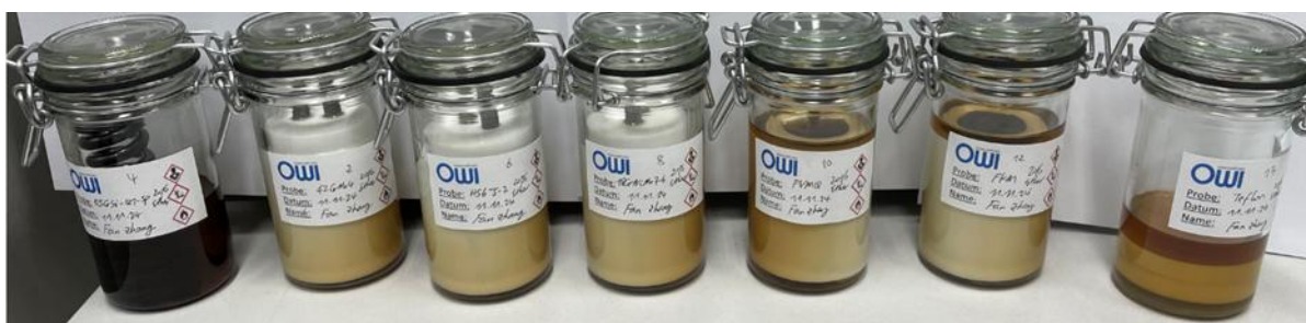
Figure 3-1 Overview of immersion test containers at start
