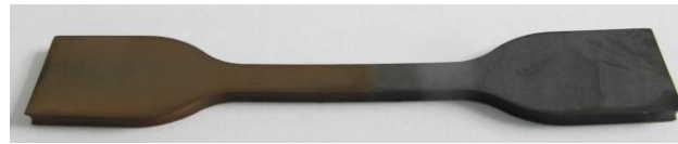
Figure 3-15 FKM before (left) and after (right) BigOxi testing in 20% ether surrogate (left fuel-immersed, right vapor-exposed section).
