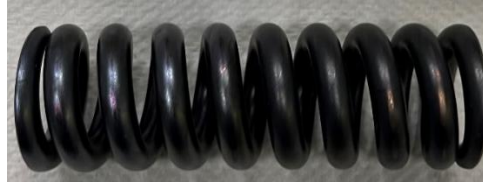
Figure 3-4 W-FA-55SiCr-QT-SP with increasing immersion time in 10% (left) and 20% (right) ether surrogate (left fuel-immersed, right vapor-exposed section).
