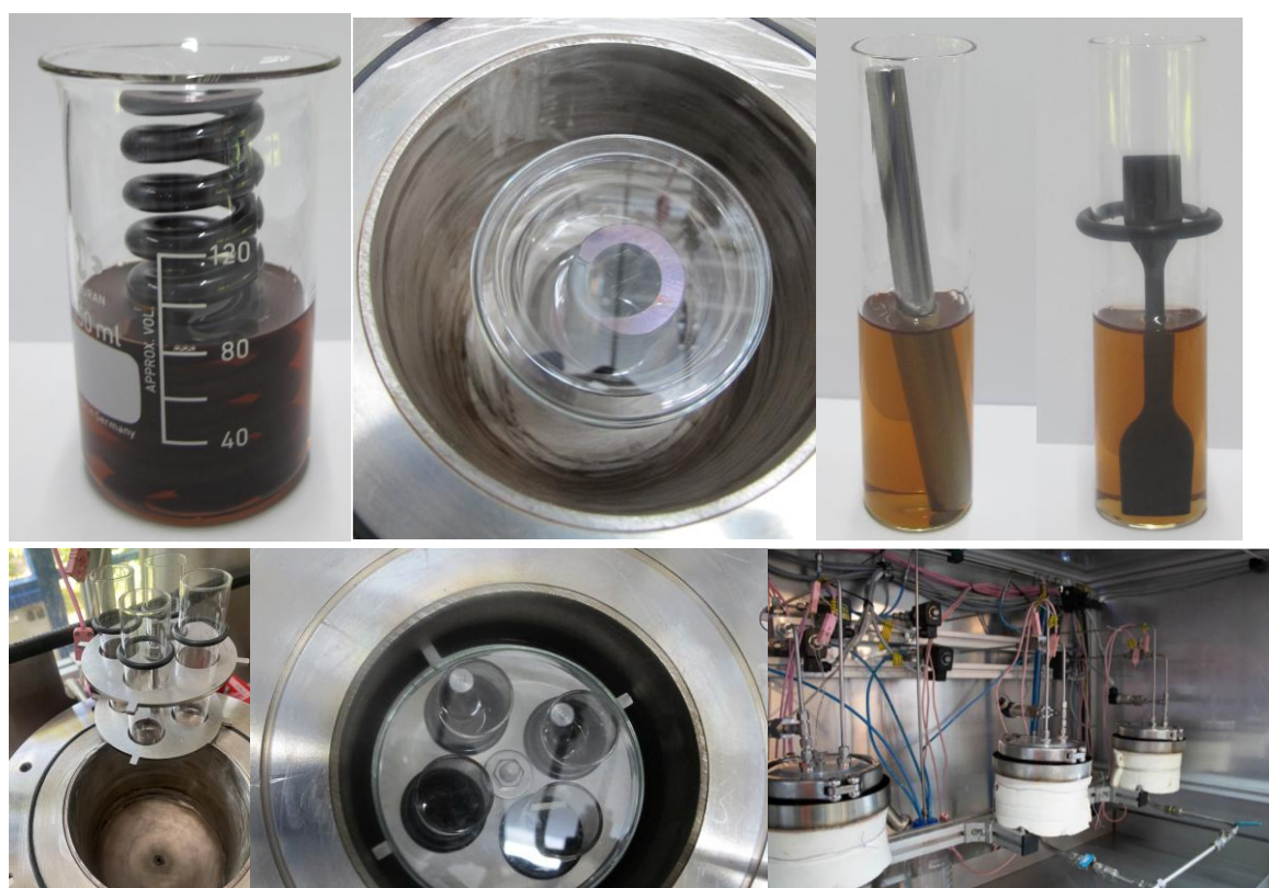
Figure 2-2 Overview of BigOxi reactors and preparation of the different sample materials inside the reactors.
