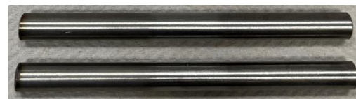
Figure 3-5 HS6-5-2 with increasing immersion time in 10% (left) and 20% (right) ether surrogate (left fuel-immersed, right vapor-exposed section).
