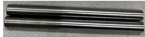
Figure 3-6 18CrNiMo7-6 with increasing immersion time in 10% (left) and 20% (right) ether surrogate (left fuel-immersed, right vapor-exposed section).
