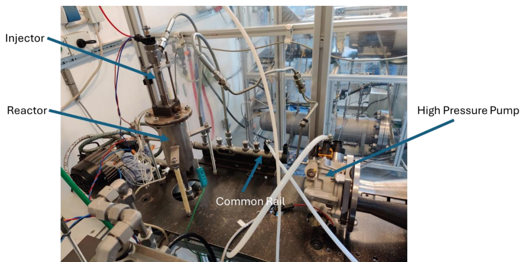
Figure 3-23 Hardware in the Loop-Testbench used for the injection system evaluation for the different blends.
