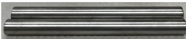
Figure 3-5 HS6-5-2 with increasing immersion time in 10% (left) and 20% (right) ether surrogate (left fuel-immersed, right vapor-exposed section).
