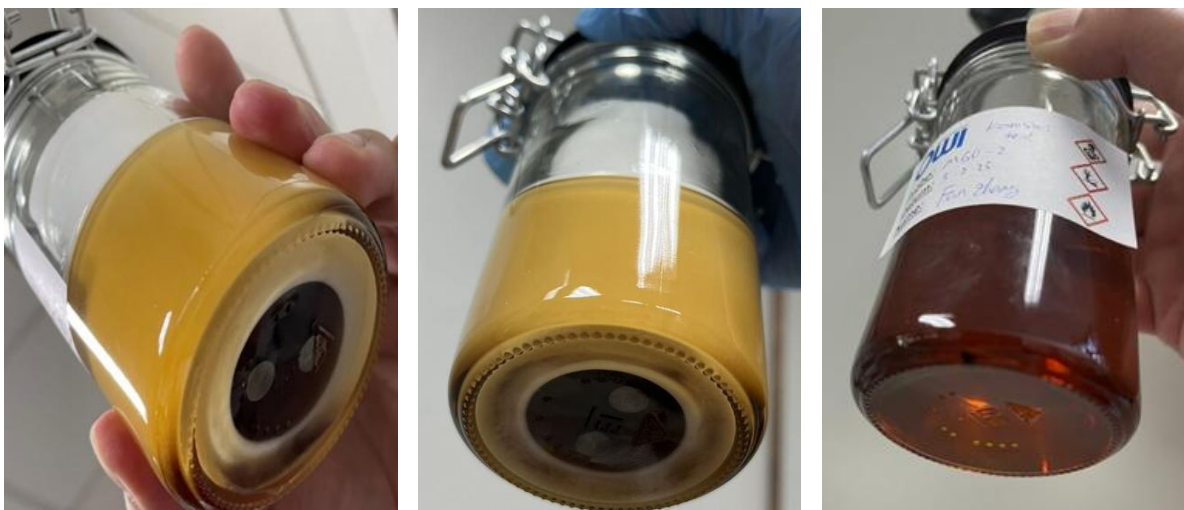
Figure 3-2 Deposits on container bottom during monthly inspection, container 1, 6 and 14.
