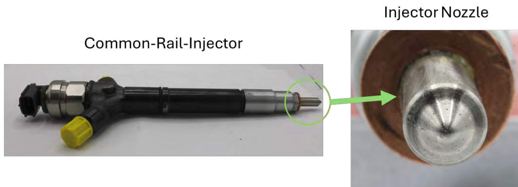
Figure 3-24 Common-rail injector and injector nozzle used for the HiL-tests.
