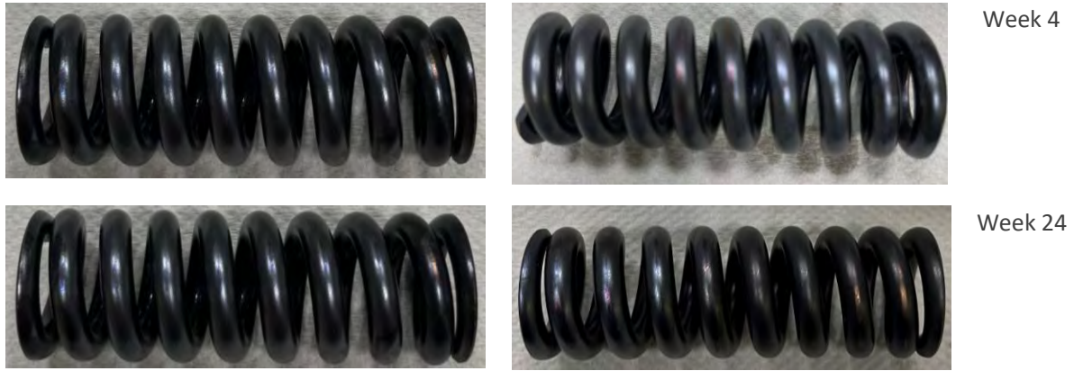
Figure 3-4 W-FA-55SiCr-QT-SP with increasing immersion time in 10% (left) and 20% (right) ether surrogate (left fuel-immersed, right vapor-exposed section).
