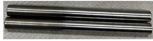
Figure 3-6 18CrNiMo7-6 with increasing immersion time in 10% (left) and 20% (right) ether surrogate (left fuel-immersed, right vapor-exposed section).
