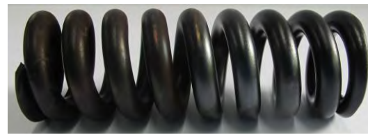
Figure 3-11 W-FA-55SiCr-QT-SP before (left) and after (right) BigOxi testing in 20% ether surrogate (left fuel-immersed, right vapor-exposed section).
