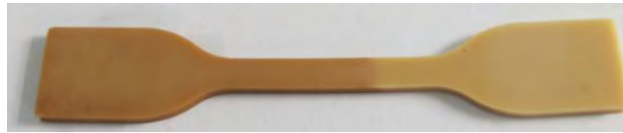
Figure 3-16 FVMQ before (left) and after (right) BigOxi testing in 20% ether surrogate (left fuel-immersed, right vapor-exposed section).
