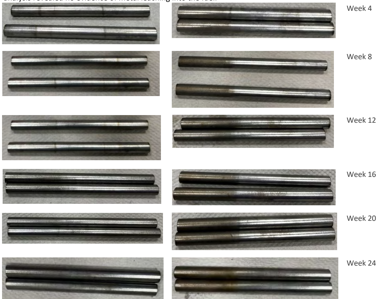
Figure 3-3 42CrMo4 with increasing immersion time in 10% (left) and 20% (right) ether surrogate (left fuel-immersed, right vapor-exposed section).
